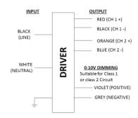
Input lead wires are 18AWG 105C/600V stranded copper with flag terminals per UL1452.
